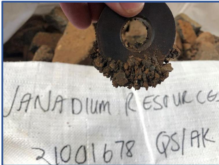
Photo 2 – Highly magnetic material contained in bulk samples
