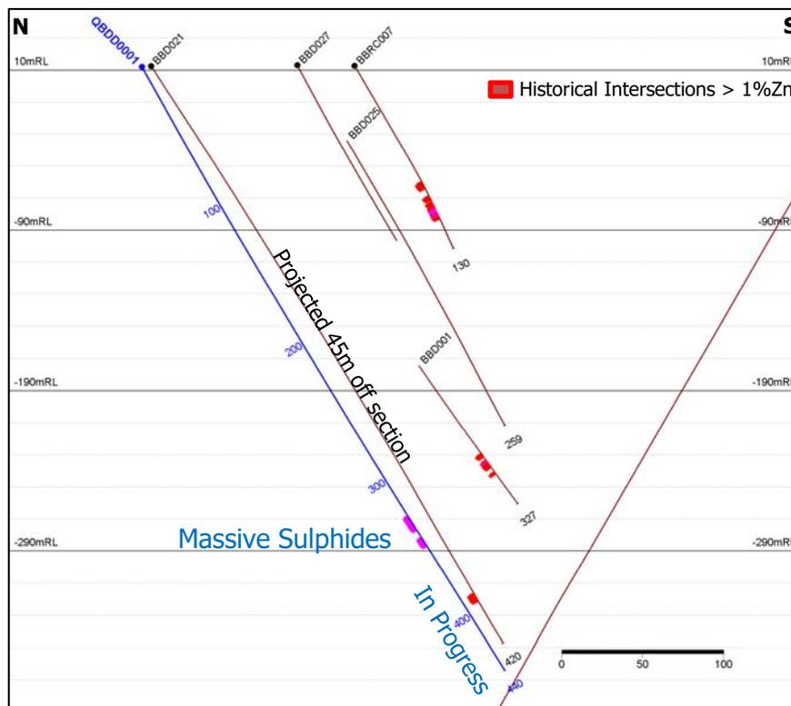
Figure 4. Cross Section View showing QBDD0001 and historical results. Note historical drilling has been projected from off section.
