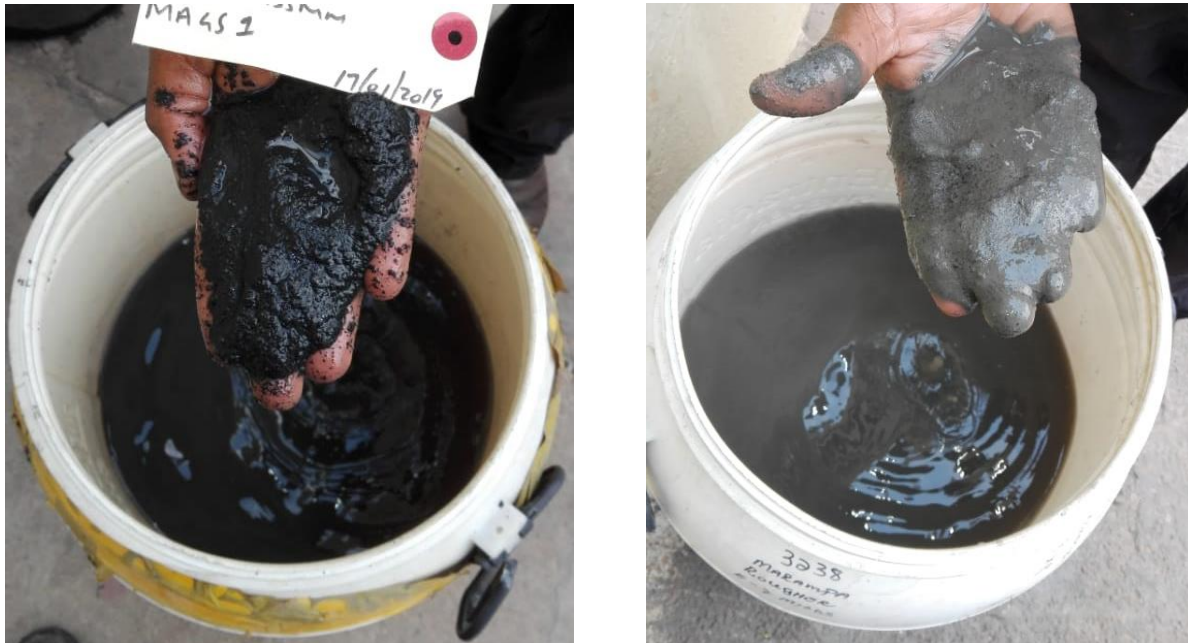
Figure 1. Examples of magnetic (LH) and non-magnetic (RH) products from magnetic separation testwork (wet). Note analyses are awaited. Samples were taken from VDD003
