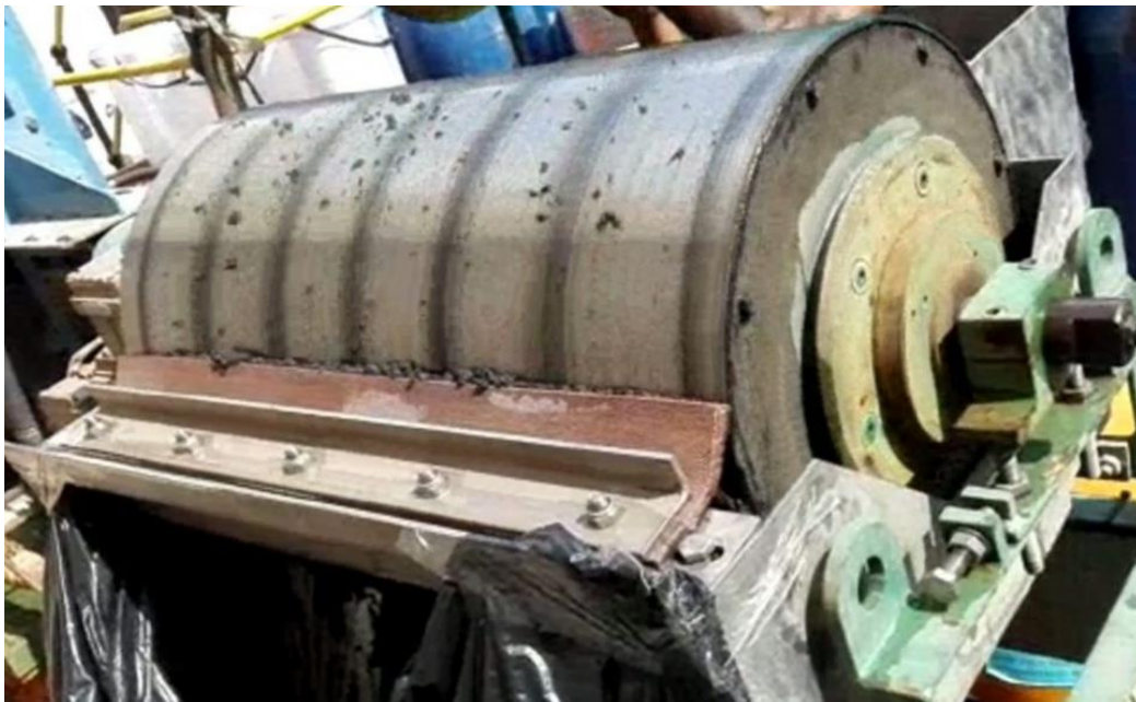
Figure 2. Magnetic separation drum used in plant simulation testwork.
