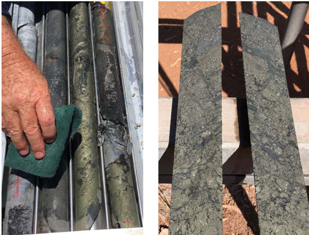
Figure 3. Images of sulphide minerals in drill core from QBDD0001 (LHS, approximately 342m downhole) and QBDD0004 (RHS, approximately 206m downhole).
