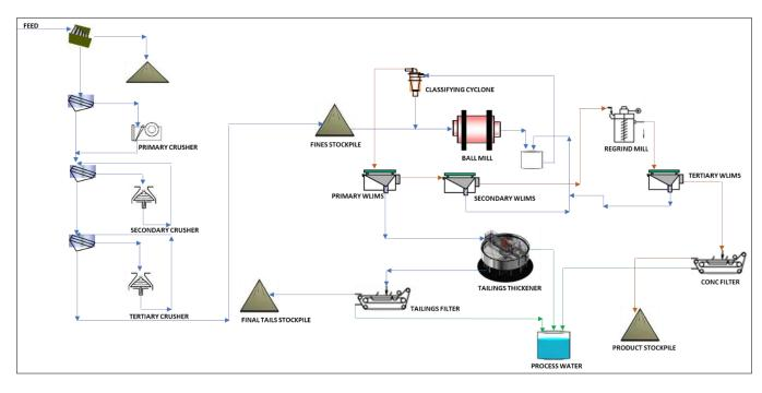
Figure 6: Concentrator block flow diagram
