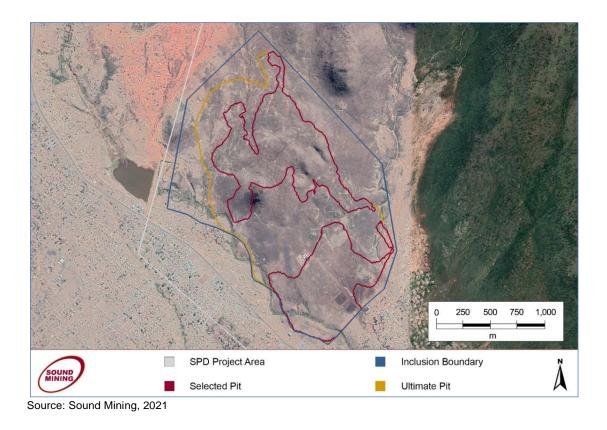
Figure 4: Plan View of Selected Pit Shell and Ultimate Pit Shell
